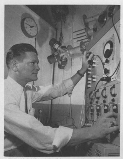
CONTROL BOARD of Sandia's new experimental plane wave sound testing facility is checked out by C. W. Remaley (1613), designer of the facility. In the background are four "drivers" which can subject materials to vibrations from 300-7500 cycles per second.
